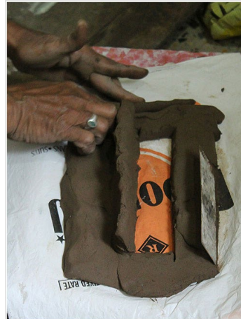
Rectangular walls being built along the edges of the cavity.
