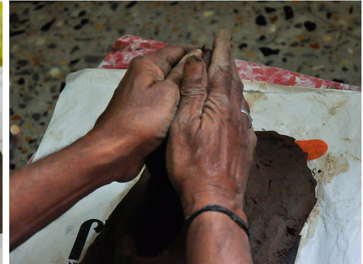
Making a hollow inside, the outline of the model is covered entirely with clay.
