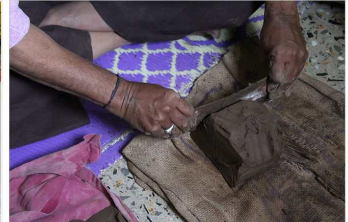
Clay is sliced into thin, flat shapes with an iron sheet.
