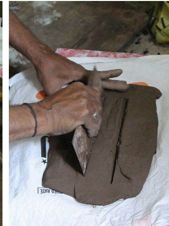
A sheet of iron is used to cut slits on the surface of the clay.
