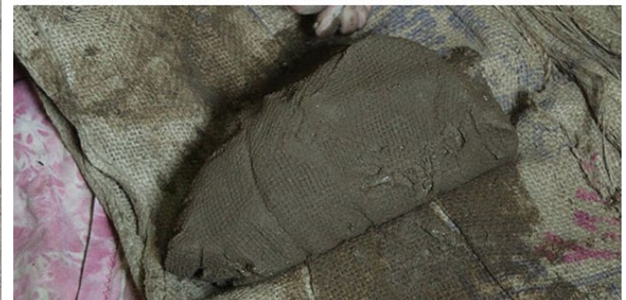
A jute sac is wrapped around the clay to absorb excess water from the clay.
