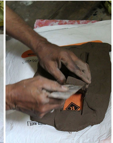
A sheet of iron is used to cut slits on the surface of the clay.
