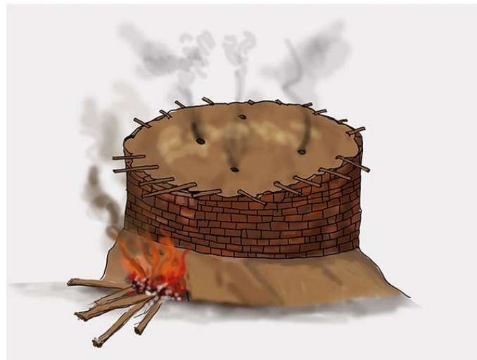
The models being subjected to a heating process in a furnace for hardening.
