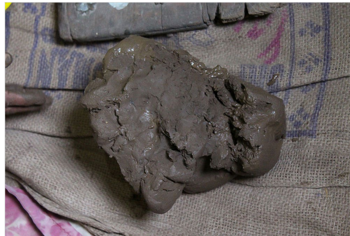
The clay is mixed with an appropriate amount of water to make it smoother and its handling easier.
