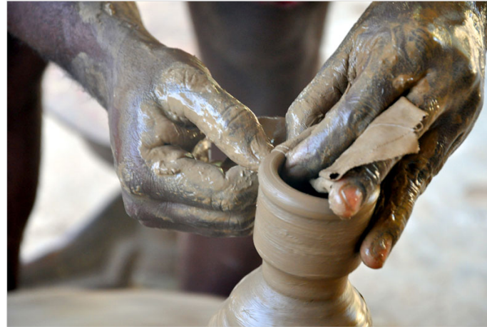
Final cleaning of object using wet cloth.
