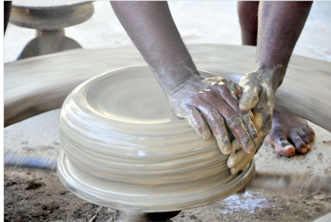
Once the wheel starts rotating, the craftsmen start to shape the clay.
