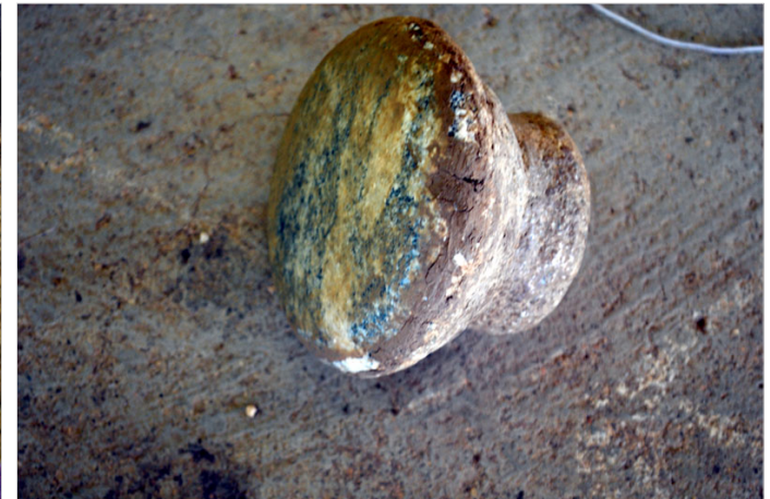
Raayi-A mushroom shaped stone which is used to beat the inner surface of objects.
