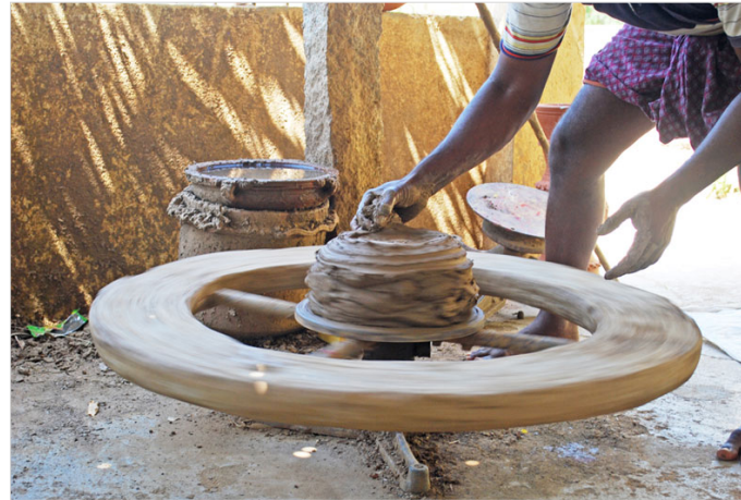
As the wheel rotates, the excess clay is removed.
