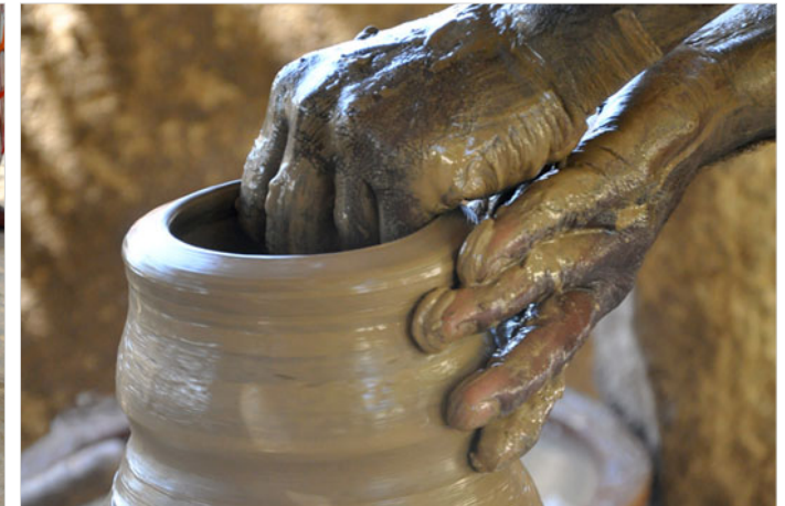
The neck of the pot is being shaped.
