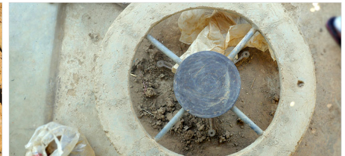
Potter's wheel made of cement.
