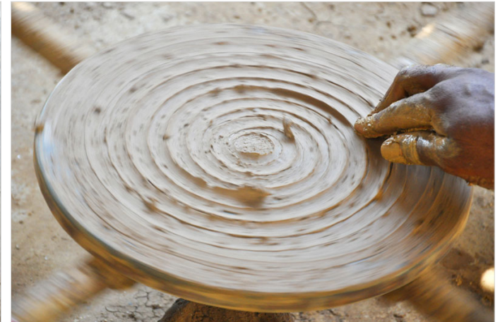
The mud is applied on the center of wheel which acts as an adhesive.
