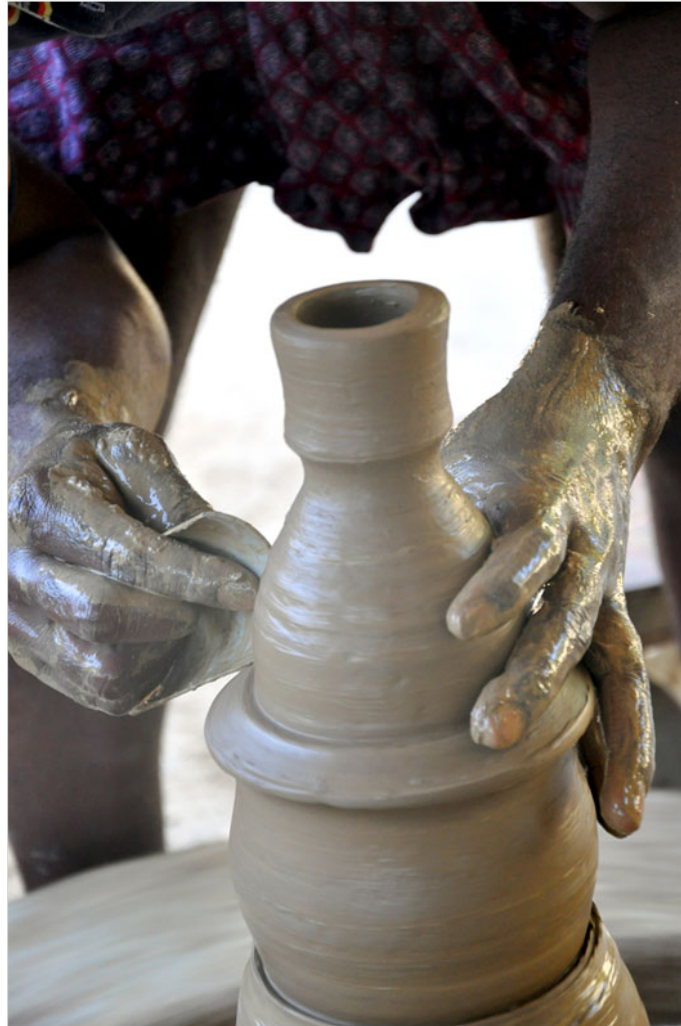
The outer surface is textured while the wheel is in motion.
