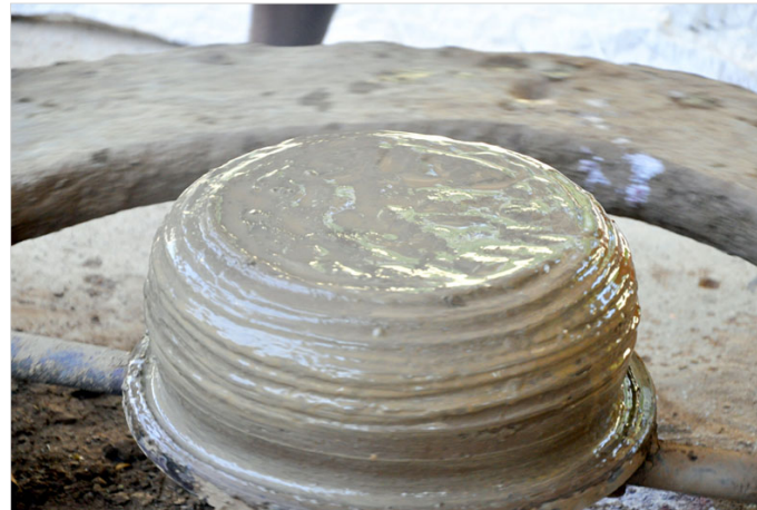
Water is applied before starting the shaping process.
