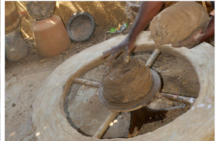
Placing the clay on the center of the wheel.
