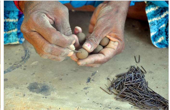
U-shaped iron sticks are inserted into the clay balls and attached to products as accessories.
