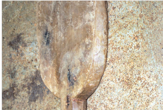
Salapa-wooden bat is used to beat the outer surface of the pot.
