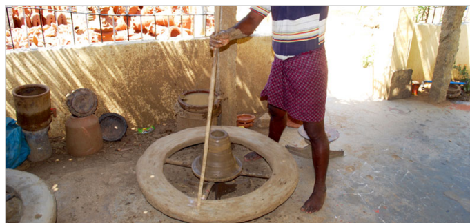
Veduru karra-bamboo stick used to rotate the wheel.
