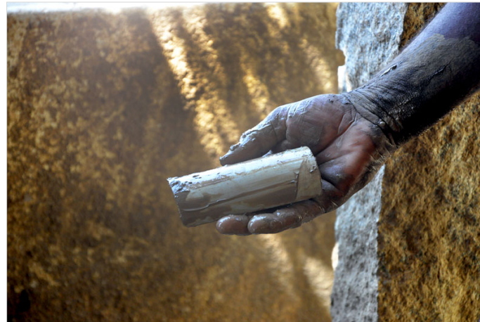
Semicircular piece of plastic used for texturing the surface of the object.
