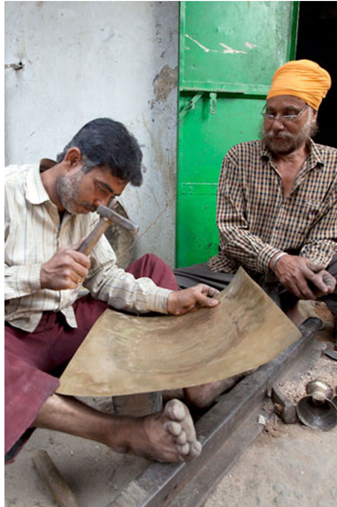
The sheet is beaten before bending it.
