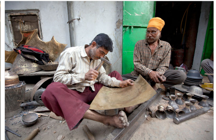
The sheet is beaten before bending it.
