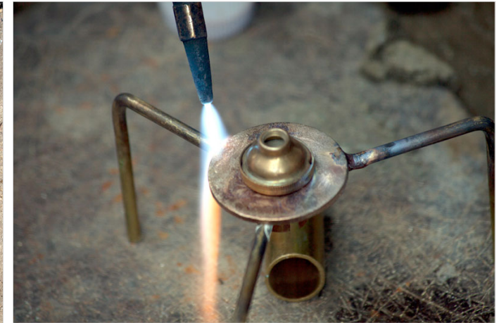
Welding machine/burner used to attach two metal pieces.
