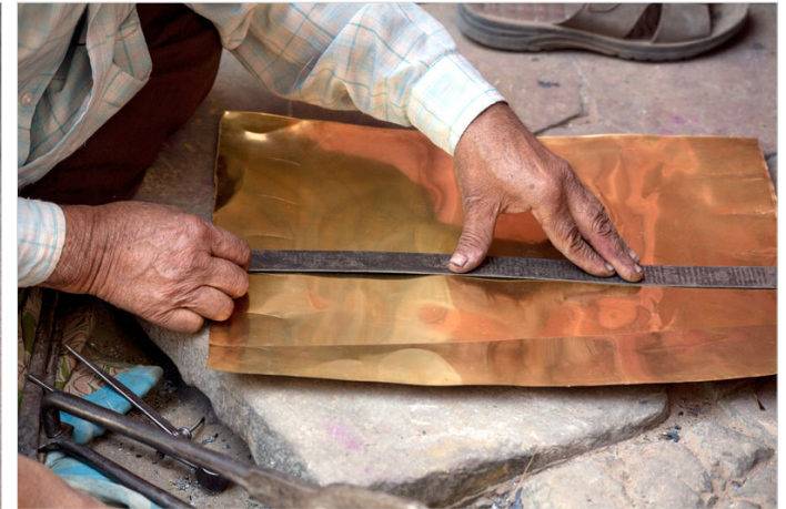
Scale is used to mark lines on the metal sheet accurately.
