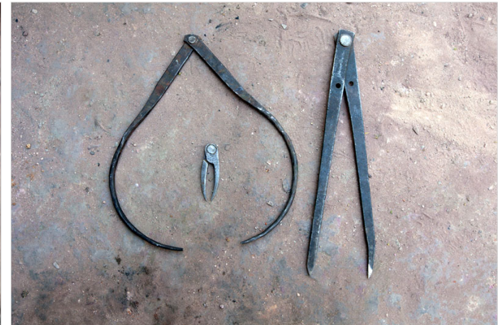
Prakaar (Compass) - Used for marking on the metal sheet.
