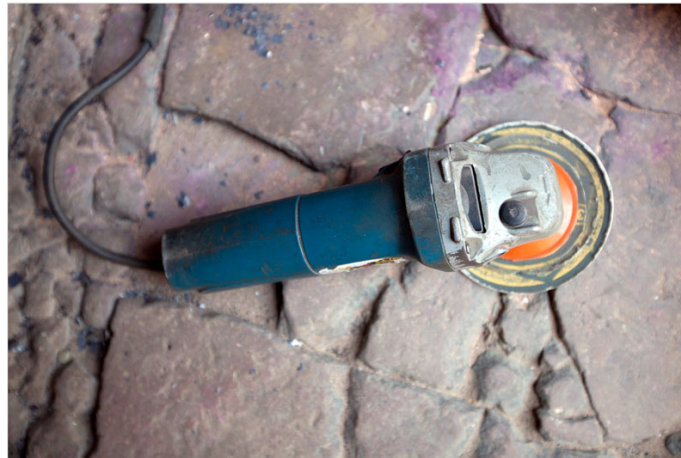
Cutting machine is used to remove the excess metal after welding process.
