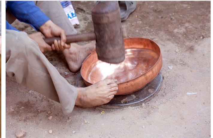
Concurrent use of legs and hands is done while hammering the metal product-in-process.
