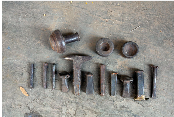
Cheni (Chisel) - Different shapes of chisels.
