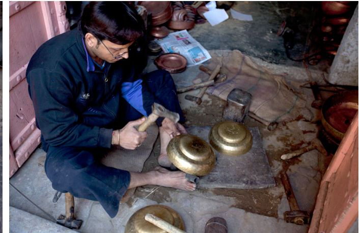
Artisan giving form and texture to a product with the help of hammer.
