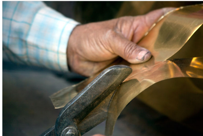
The metal sheet is being cut with the help of metal scissor.
