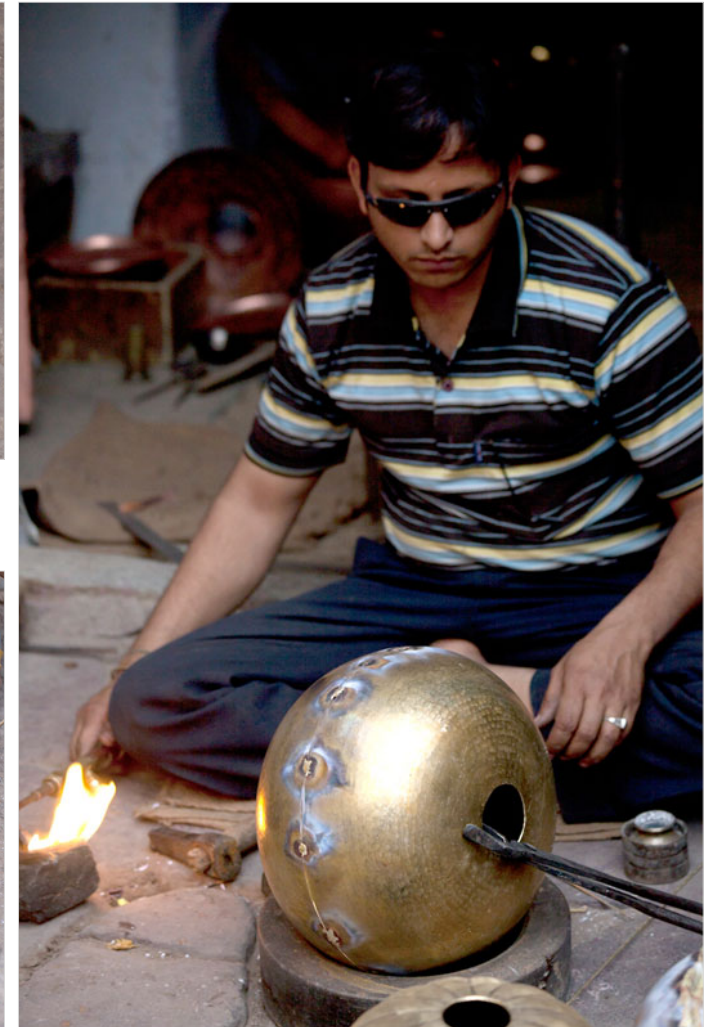
Two parts are combined by welding.
