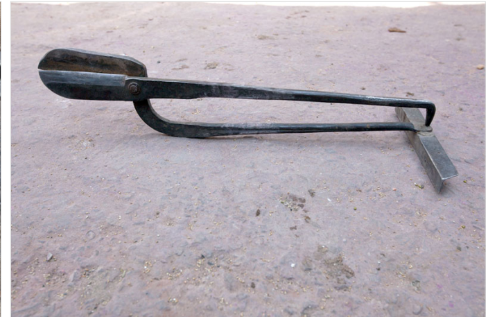
Metal Scissors used to cut the thick metal sheet.
