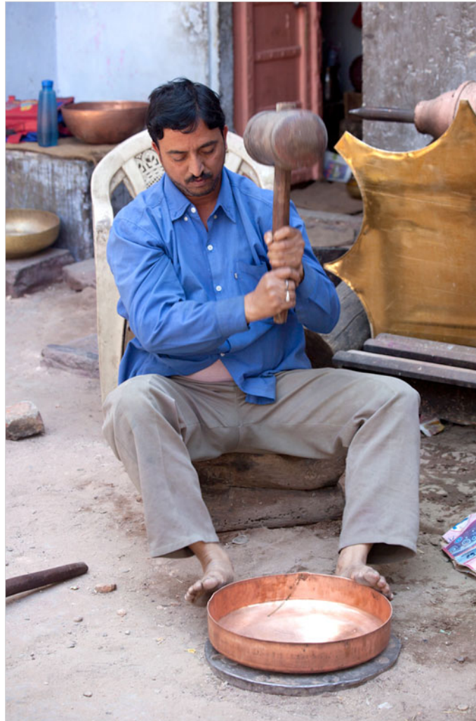
Constant hammering is done to obtain the shape of the bowl.
