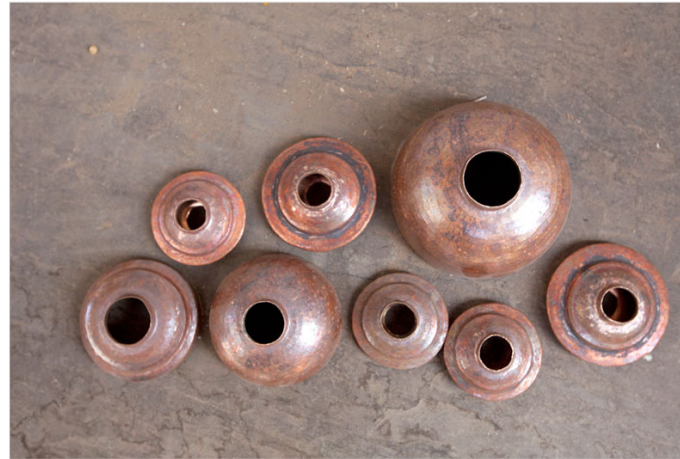
The parts of traditional Kalash are ready for welding process for joining purpose.
