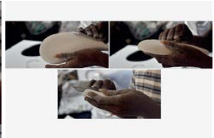
Sharp edges being curved using sandpaper.
