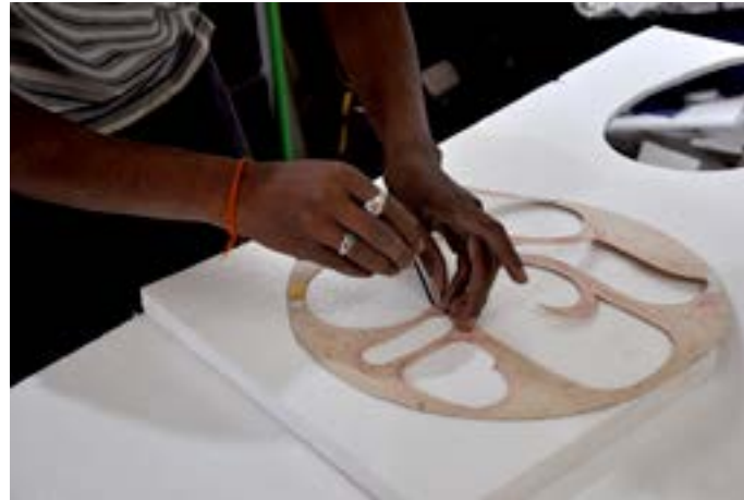
Using the stencil, markings are done for the intended model of thermocol.
