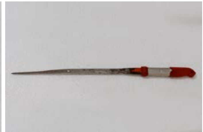
Thermocol cutter is used to cut the thermocol along the indicated marking.
