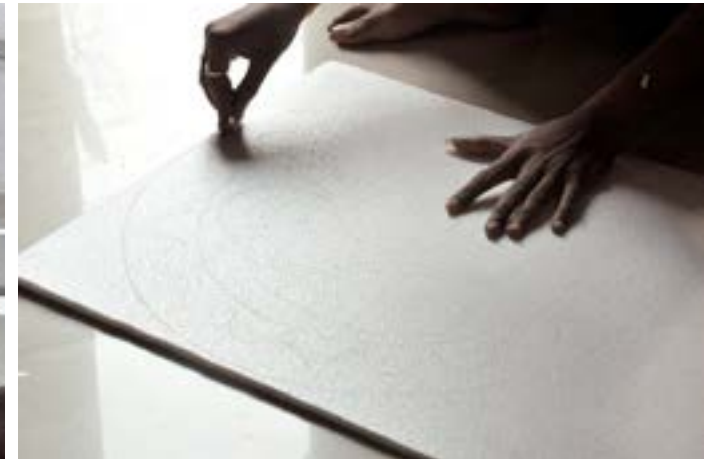
A thin sheet of thermocol being cut using a stainless blade to prevent breakage of the sheet during further processing.
