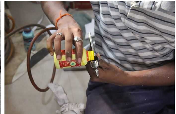
Acrylic paint is poured into a spray gun.
