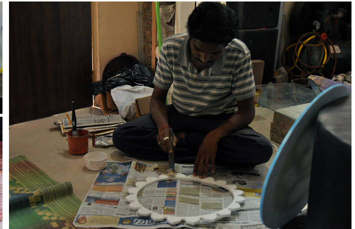
Synthetic adhesive is applied to a thermocol ring.
