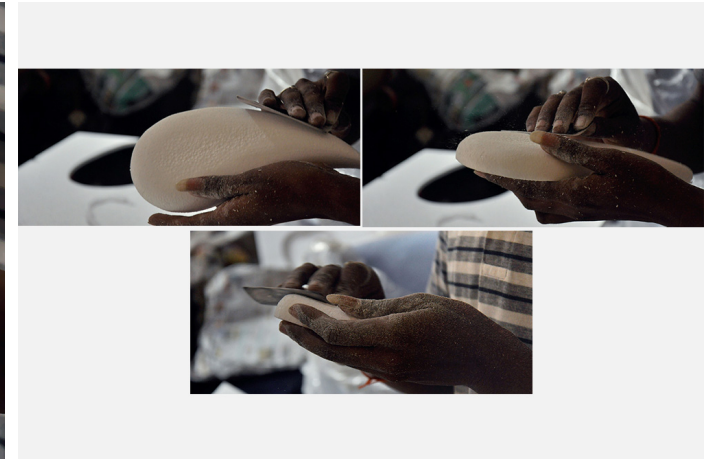
Sharp edges being curved using sandpaper.
