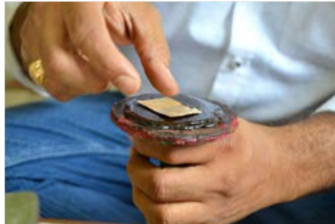
23 karat gold foil sheet being fixed on lac.
