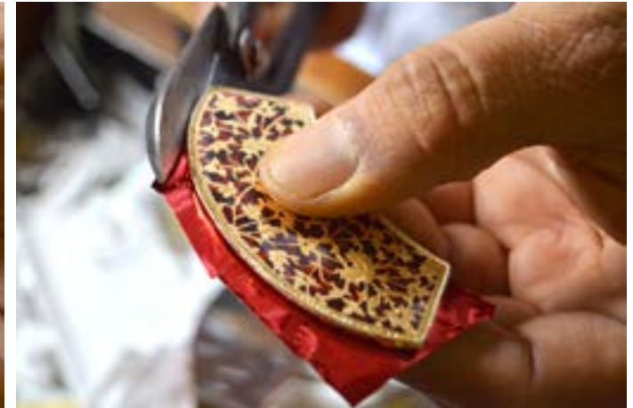
Colored foil is inserted under the glass to add brilliance.
