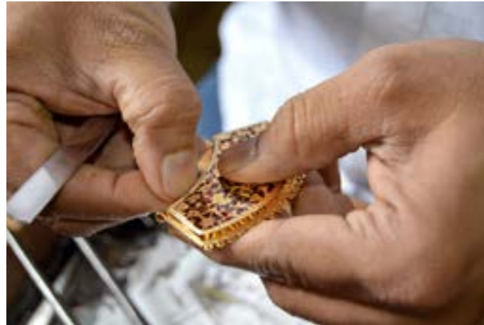
The edges of the case being closed in.
