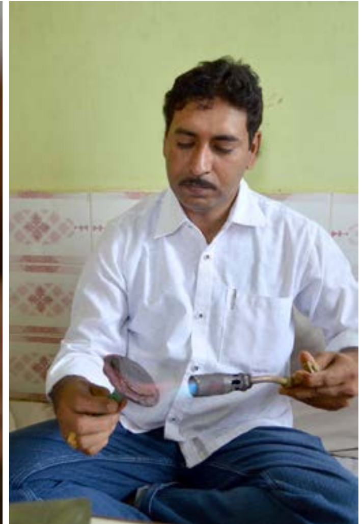
23 karat gold foil sheet being fixed on lac.
