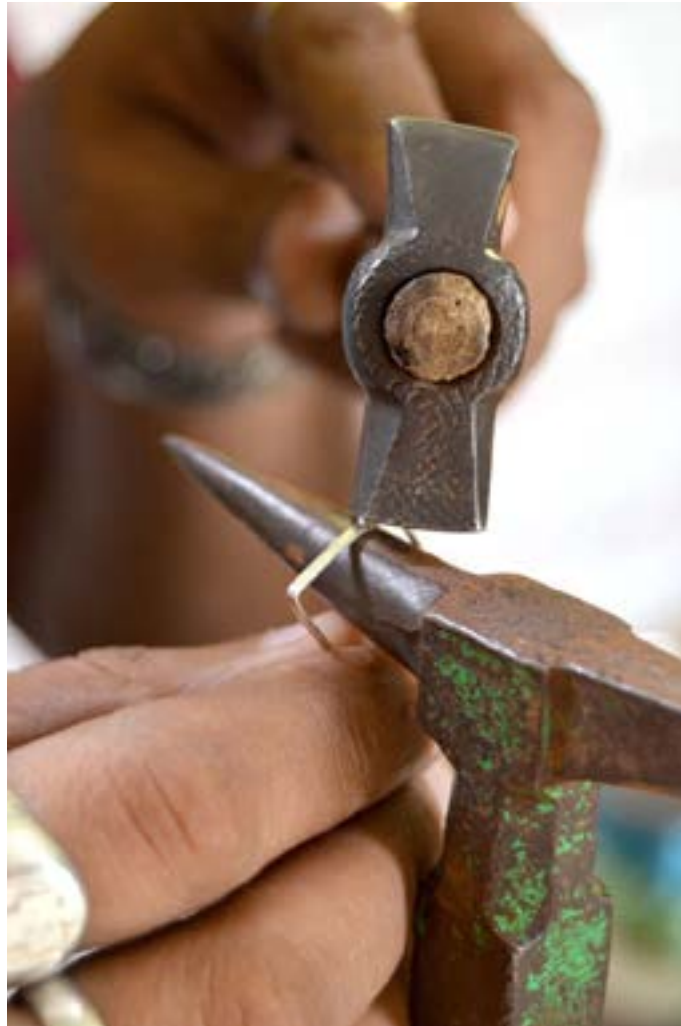
Silver strip being shaped like the glass.
