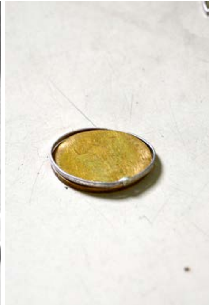
Example of how the silver strip fits on the glass (by showing it on a die).
