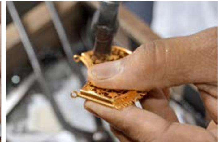
The edges of the case being softly hammered to close in over the glass.
