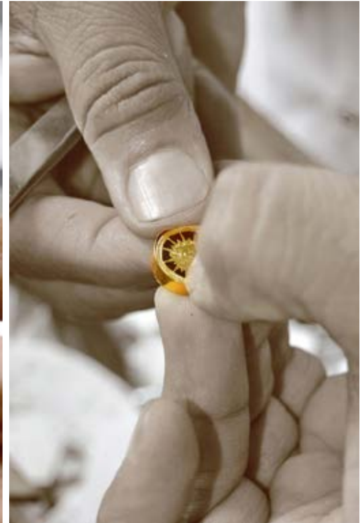
The edges of the cuff links case being softly hammered to close in over the glass.
