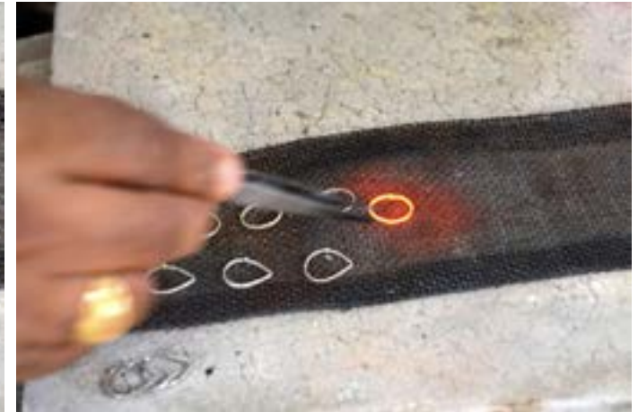
Silver strip being shaped like the glass.
