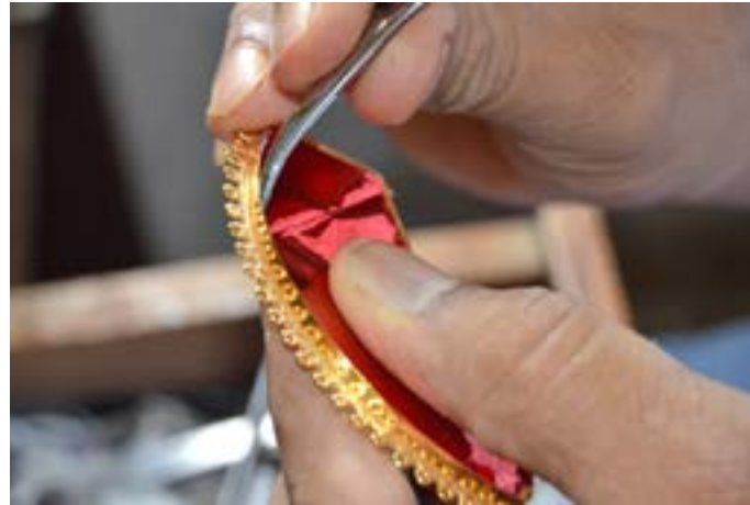
Colored foil is inserted under the glass to add brilliance.
