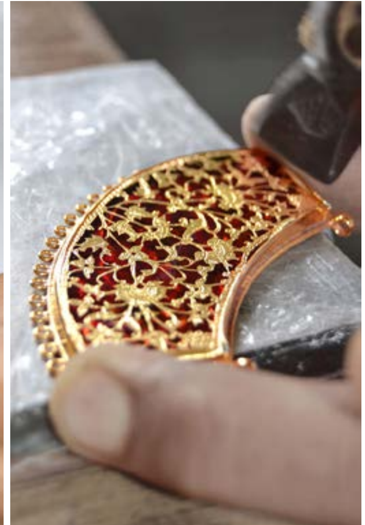
The edges of the case being softly hammered to close in over the glass.
