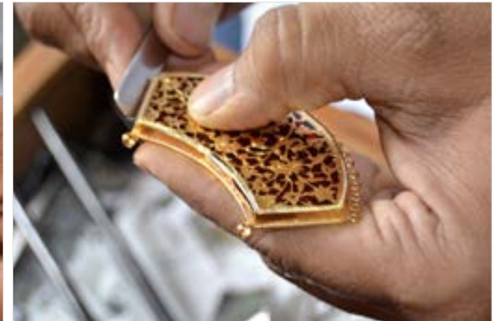
The edges of the case being closed in.
