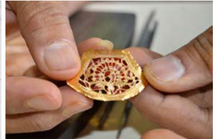
Glass cut out in the same shape as the metal foil.
