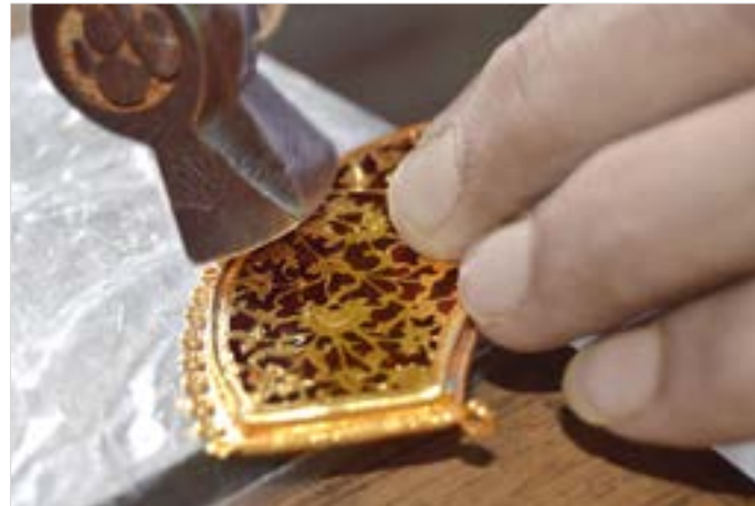
The edges of the case being softly hammered to close in over the glass.
