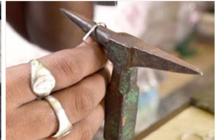
Silver strip being shaped like the glass.
