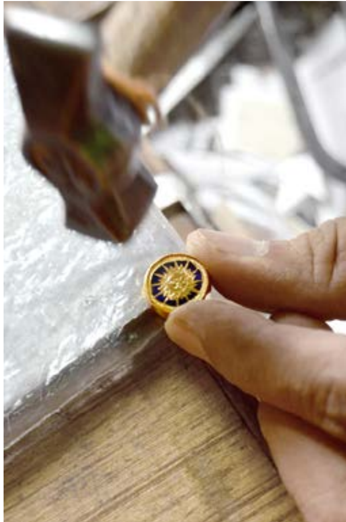
The edges of the cuff links case being softly hammered to close in over the glass.
