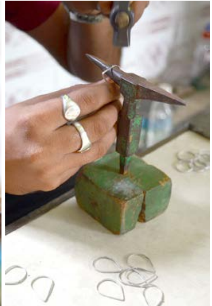
Silver strip being shaped like the glass.
