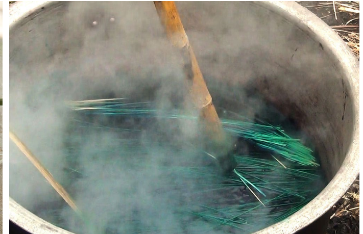
Bamboo strips dipped into the colour mixed boiling water to colour the strips.
