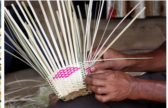
Artisan pulling the attached strips to make it tight.
