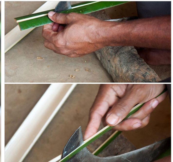
Artisan splits the bamboo into equally divided strips.
