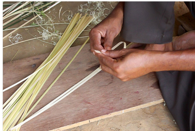
Artisan is making sure that the strips have an equal width.
