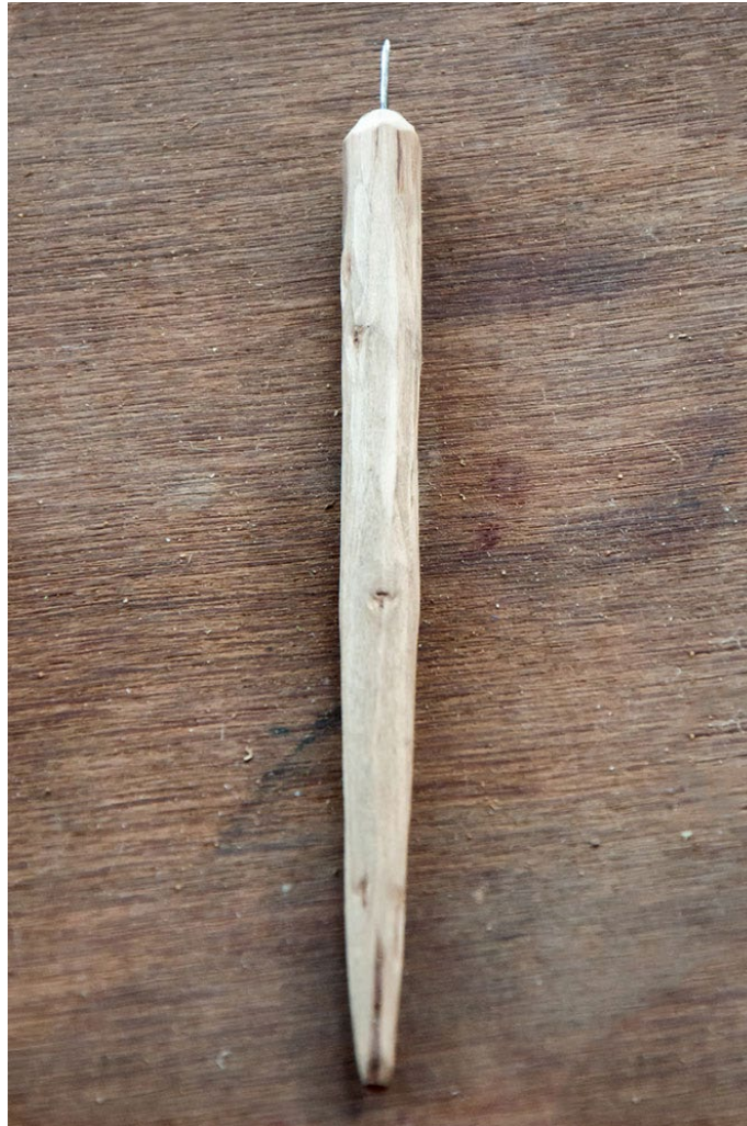
Customized needle tool is used for weaving bamboo strips on products.
