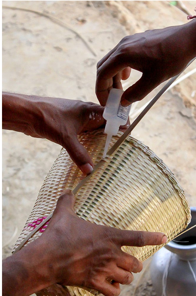
Glue is added on the intersection points where the long strip and basket collide.
