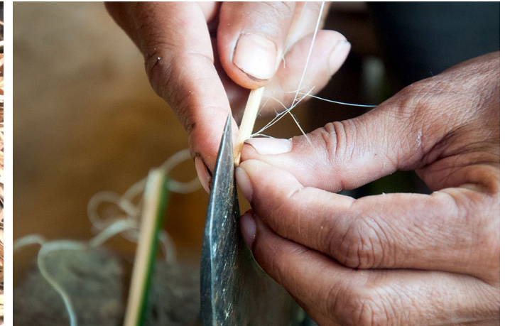
The thickness of the bamboo strip is reduced.
