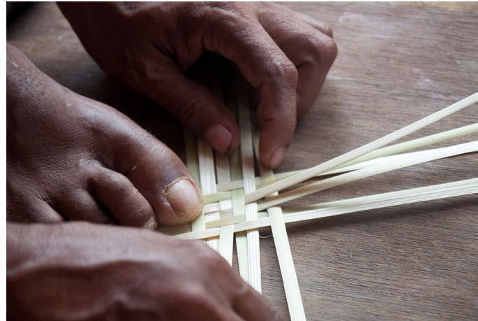
Bamboo strips are woven in a crisscross pattern.
