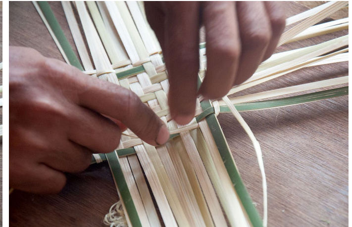
Bamboo strips with green skin are used at the edge of the base corners for strong sustainability.
