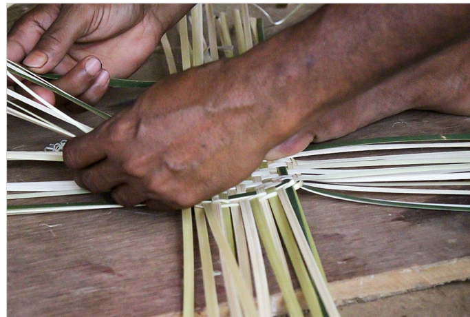
Weft strips are used to form the base sides of the basket.
