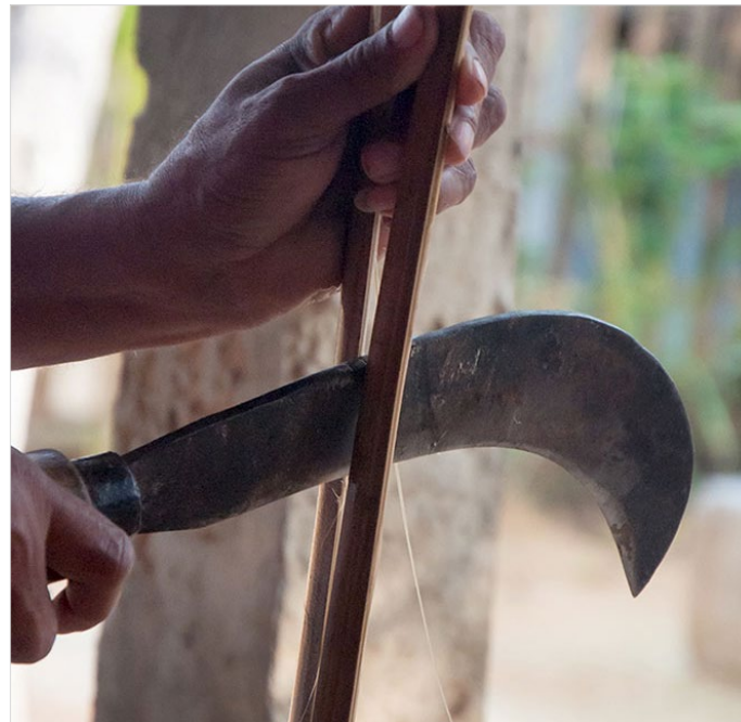
Artisan cuts the bamboo into two halves using Billhook as a cutter.
