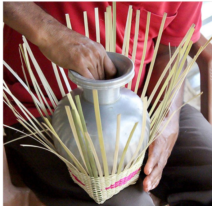
An aluminum pot is placed inside the basket to increase the width dimension.
