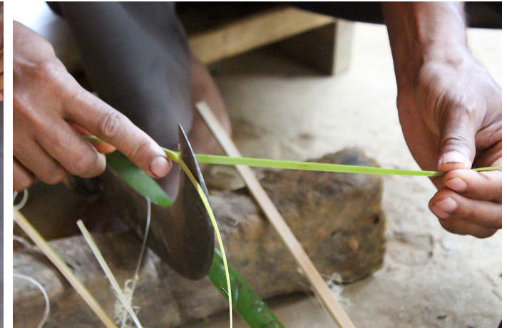
The outer skin of bamboo is removed from the strip.
