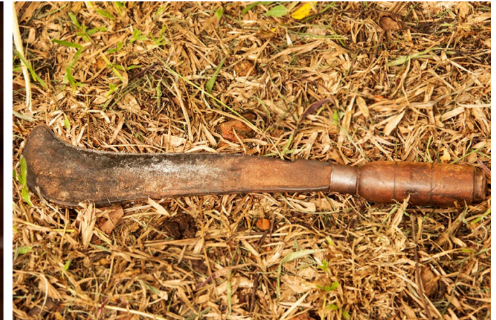
Bill Hook is used for cutting bamboo stems and for making strips from it.
