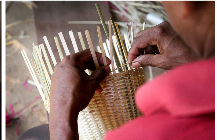
The aluminum pot is removed, and the top edge border is made.
