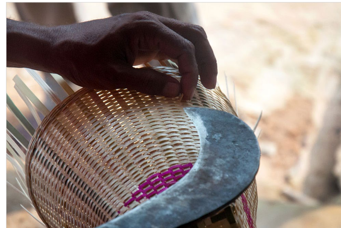
Excess strips are cut down using Billhook.
