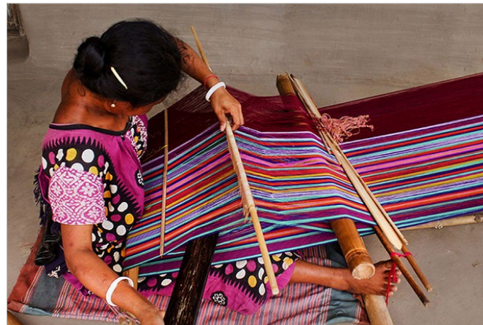
Once the fly-shuttle is passed, the artisan starts to beater to join the threads.
