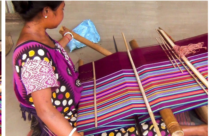
Artisan passing the bamboo fly-shuttle through the middle of the wrapped threads.
