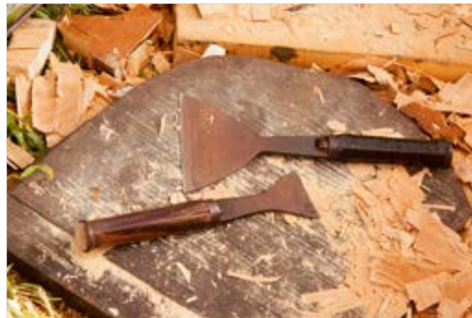
Chisels are used for chopping the wooden logs.
