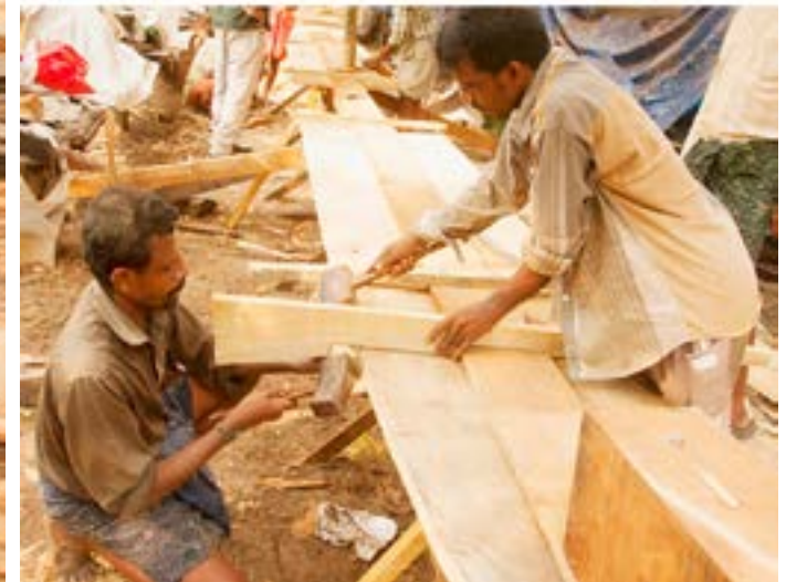
Wooden logs are arranged as per the design of the boat.
