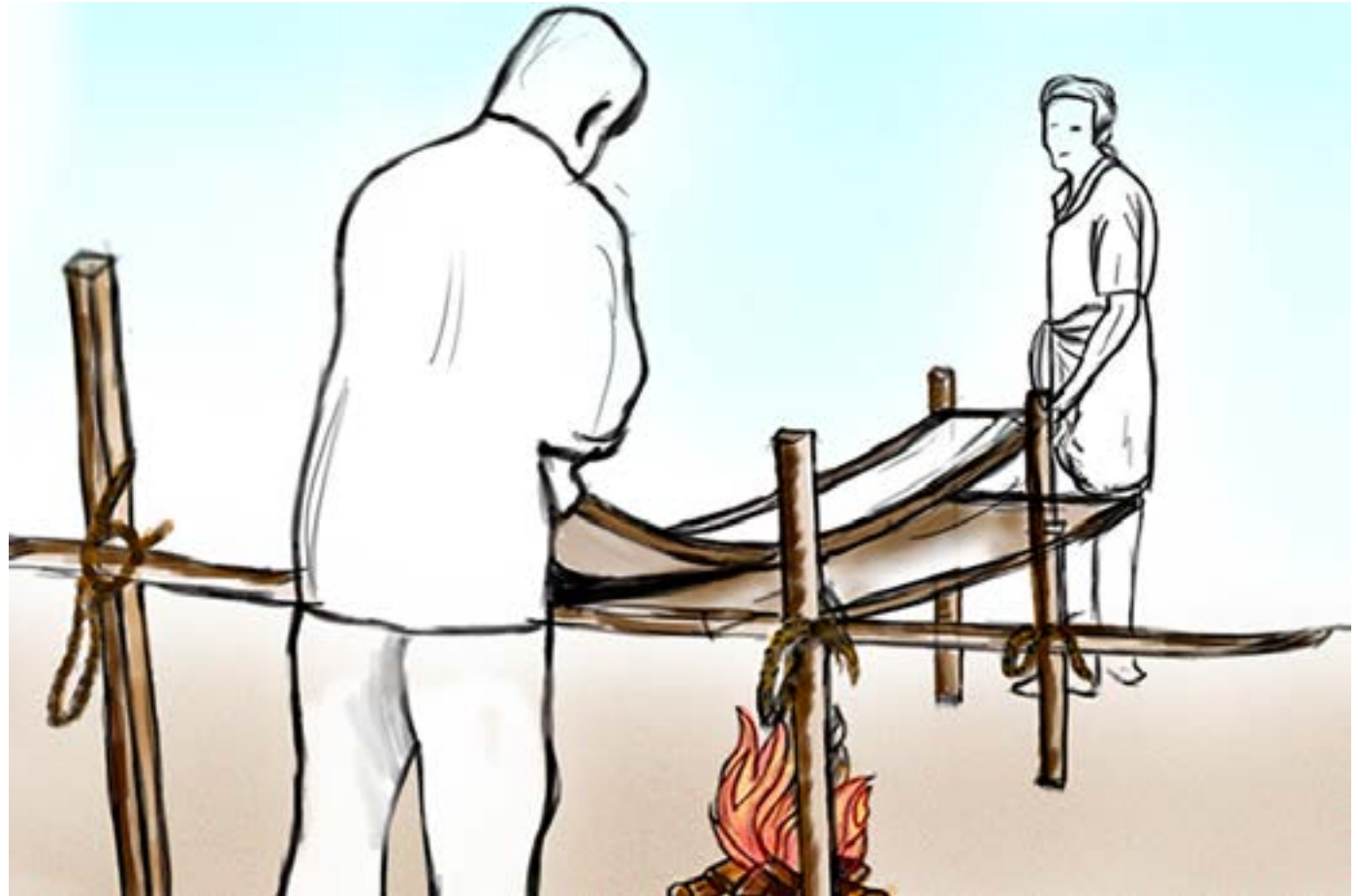
Traditionally wooden planks are mildly heated and obtained curvature of the boat.
