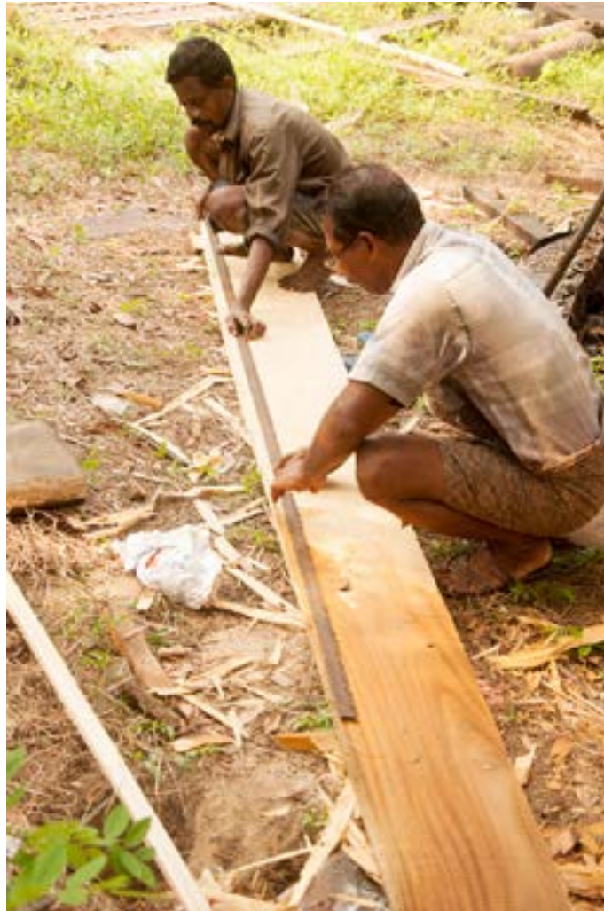
Wooden logs are measured as per the requirement.
