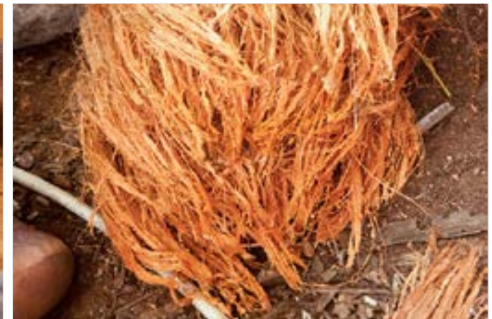
Coconut coir used for filling up the gaps in-between the planks arranged for boat making.
