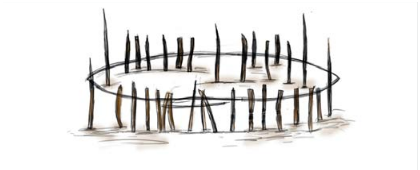
Initially wooden logs are arranged vertically on the ground.
