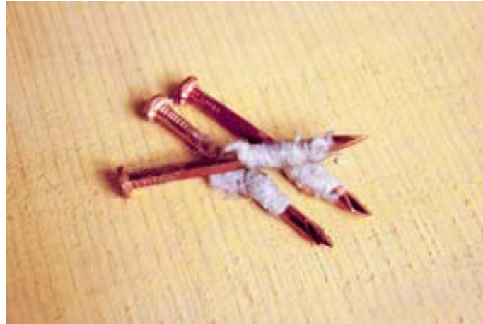
Copper nails are used for joining the wooden planks.
