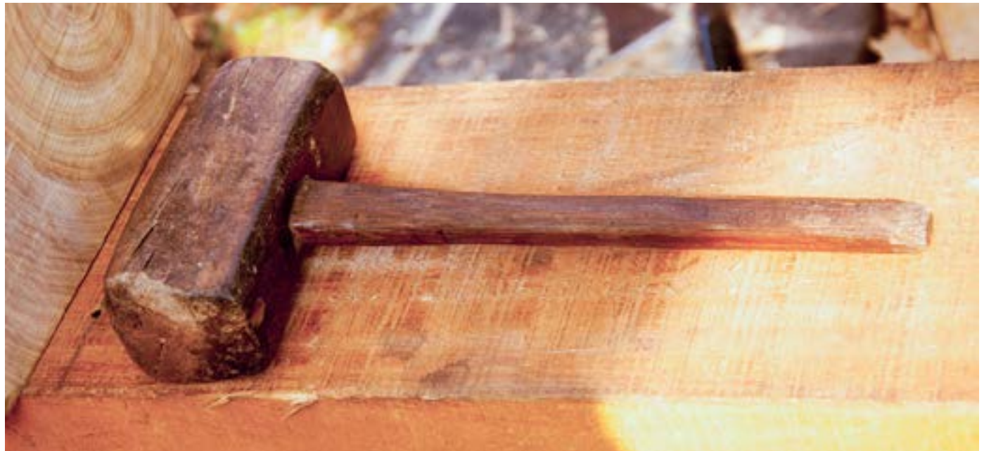
Wooden hammer used for arranging the wooden logs tightly.
