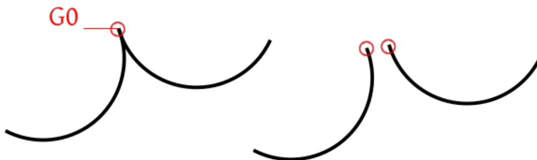
Figure 7: G^0 continuity. Curves will be continuous but there is visible stop point.
