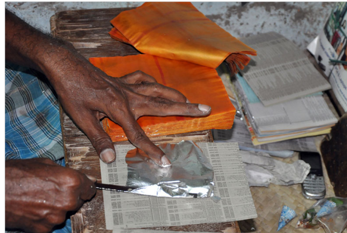
The silver foils are taken from the book and placed between the newspapers.
