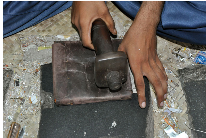
The book is covered with a leather pouch and beaten with hammer.
