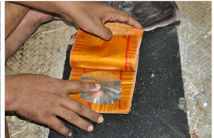
The silver pieces are converted into a silver foil.
