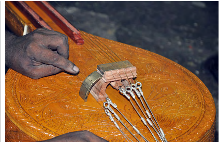
The copper strings are being placed on the bridge of the veena.
