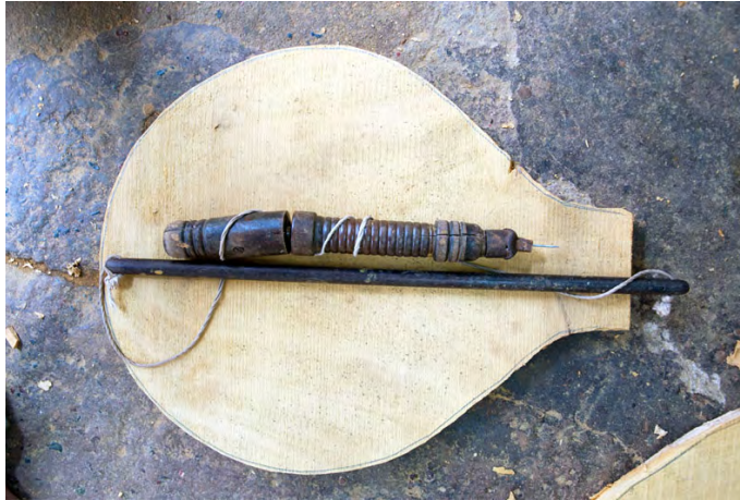
Thamur kodu – drilling machine to make holes.
