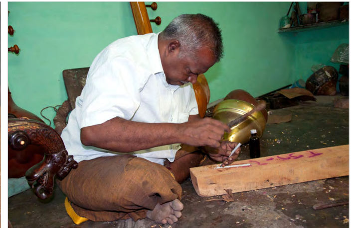
The design to be embellished is first carved on an acrylic sheet.
