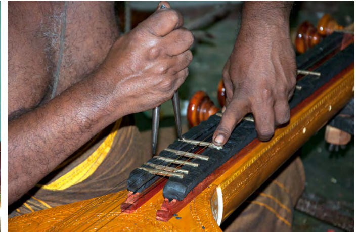
The metal frets are placed and fixed on the black dough.
