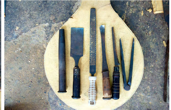
Uli- chisel, Mularam- rough chisel and small chisels.
