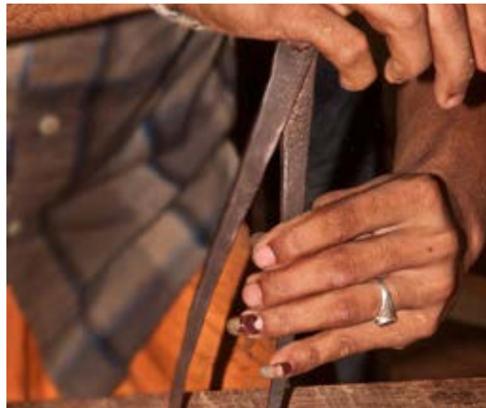
Compass is used to mark the designs at equal lengths.
