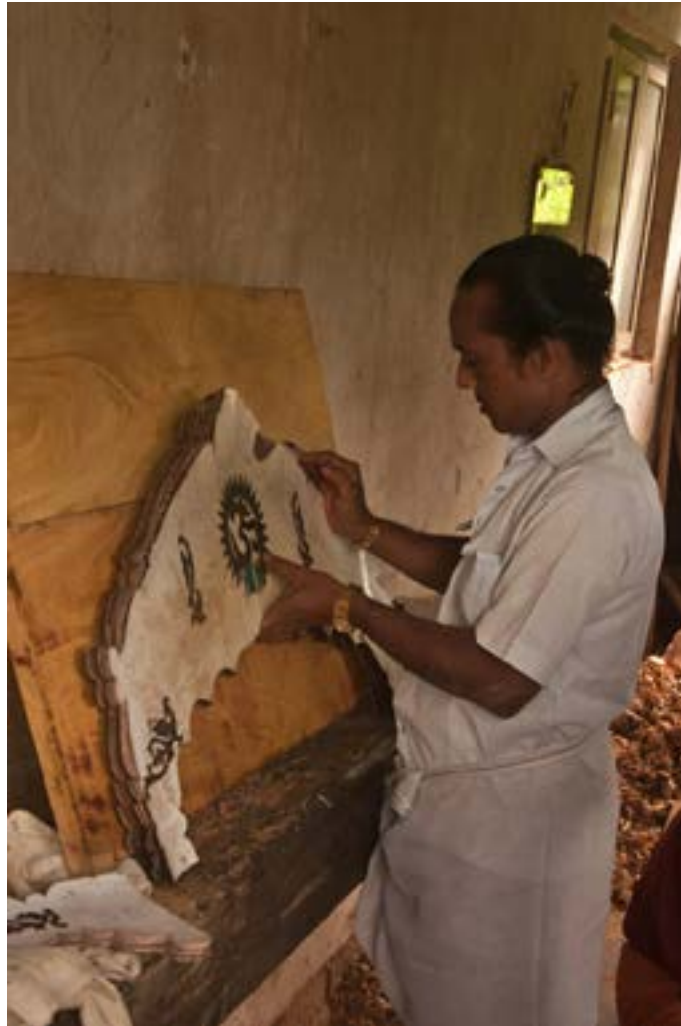
The traditional design of the door panel is being marked on the wood panel.
