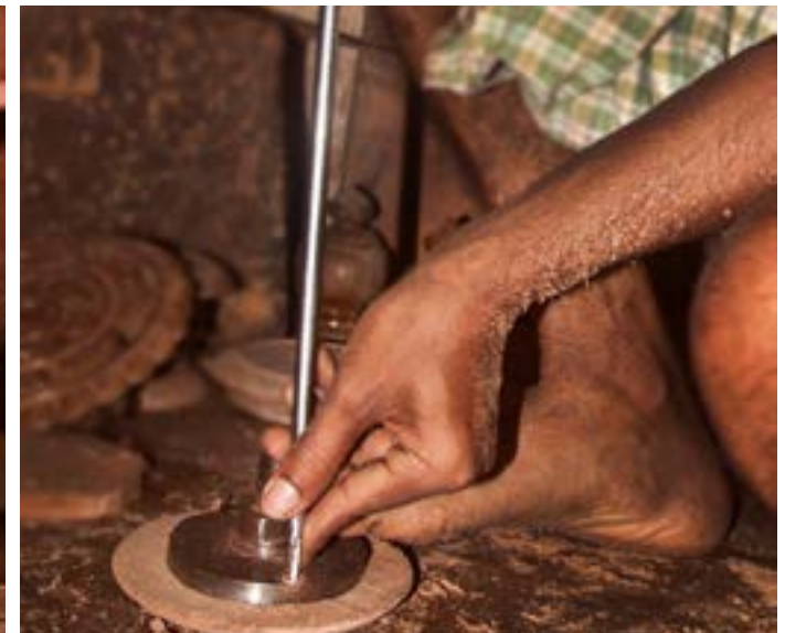
The wooden piece is being fixed to the tool of the lathe machine.
