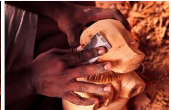
Surface is smoothened using sandpaper.
