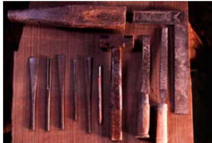
Varieties of chisels and files are used to carve the wood into desired idol.
