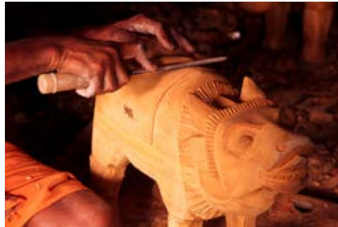
The carved articles are filed to even the surface and give a proper shape to the idol.
