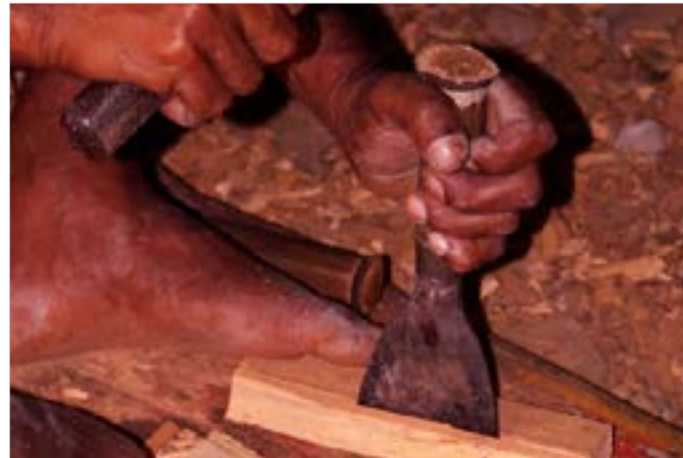
Wooden piece is inserted to join the parts together as fastener.
