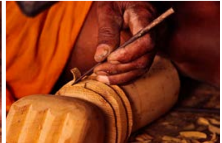
Profile or V shaped chisels are used to carve grooves
