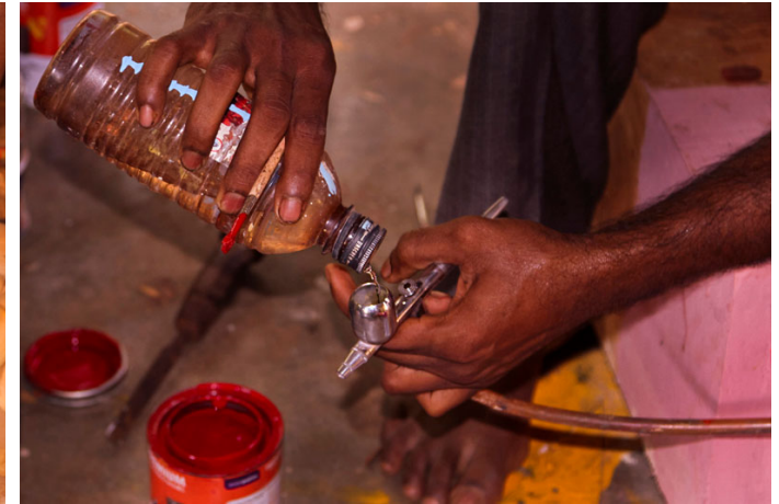
Enamel paint is used to protect and color using spray gun.
