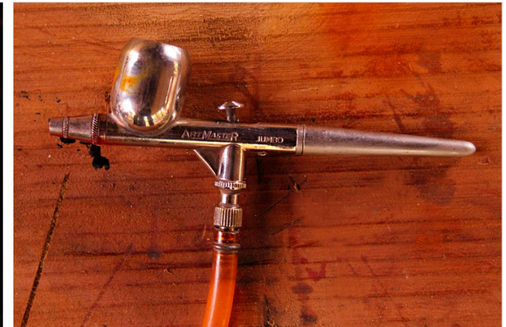
Spray gun is used to paint as it takes less time and spreads the color evenly on the surface.
