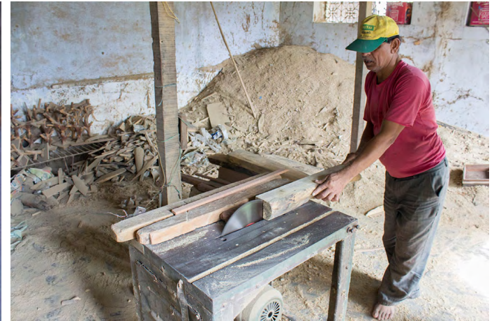
Senior artisan cutting the wood using a power saw.
