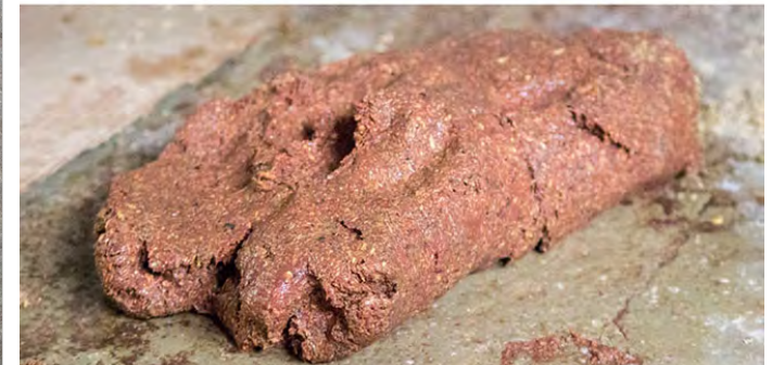
Mixture of tamarind seed paste and saw dust used to make lappam.
