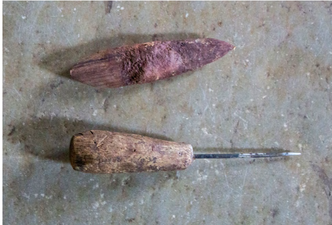
Handheld needles are used for making holes and as a sculpting tool to sculpt lappam.
