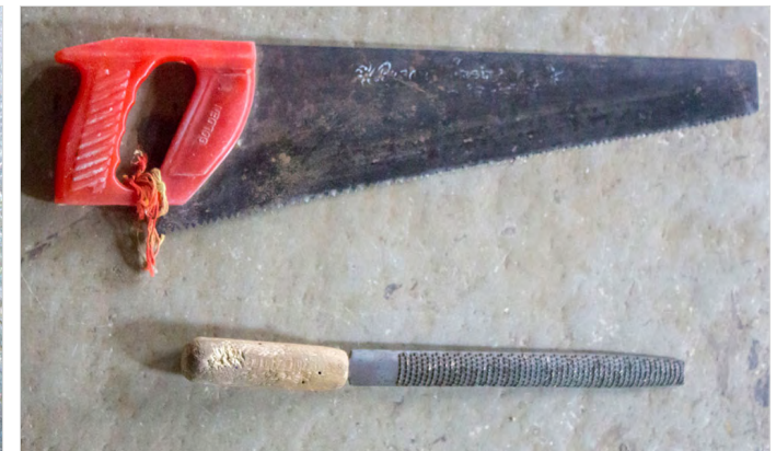
Hand saw and wood file used for cutting and shaping the wood.
