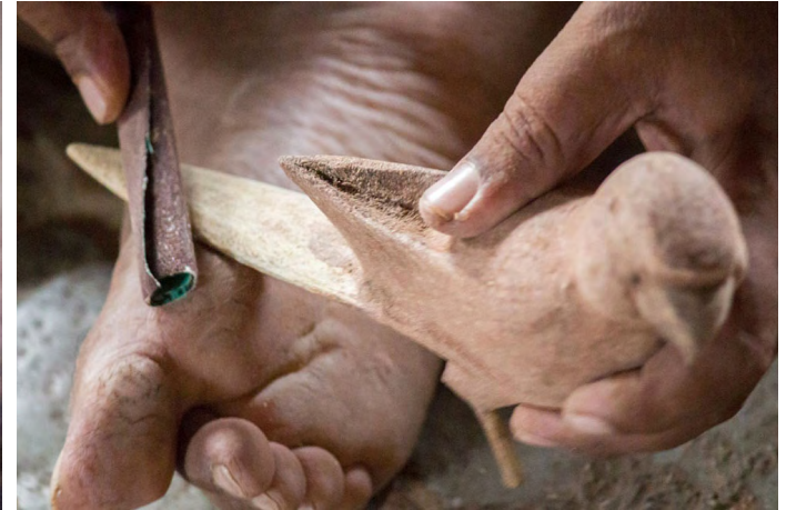
After drying rough edges are smoothened using sand-paper.
