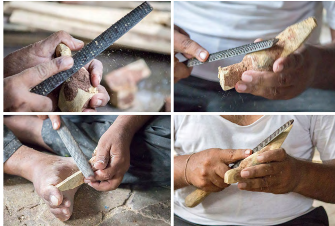
Toy is being filed to get the required shape.
