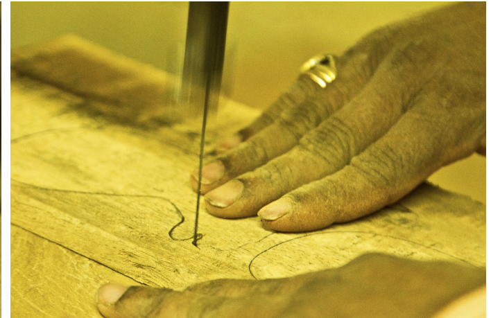
Automated thin saw blade is used to cut the wooden plank.
