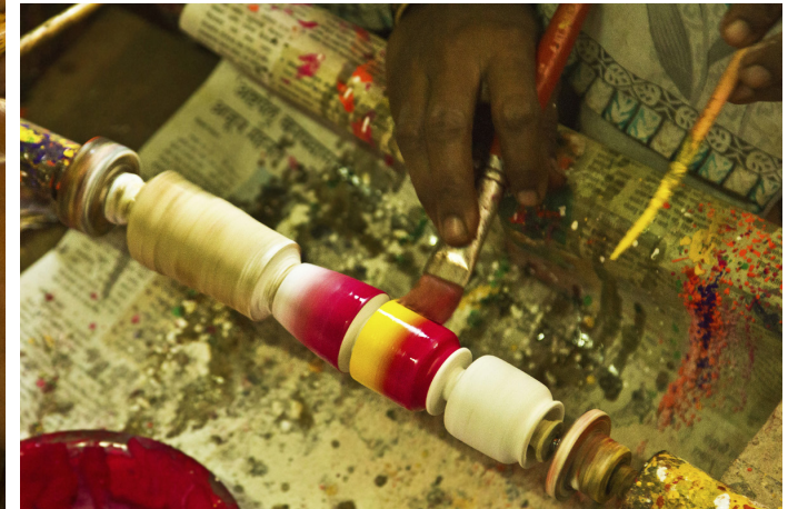
A flat brush is used to smudge two colors.
