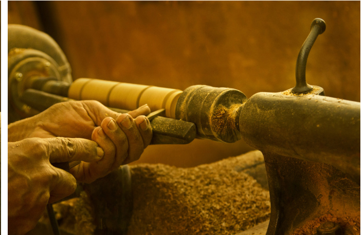
Different kinds of chisels are used to create the groves.
