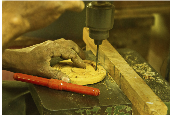
Semi-finished article is drilled as per the requirement.
