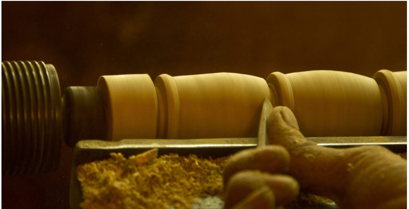
A metal rib is fixed while turning which supports the cutting tools.
