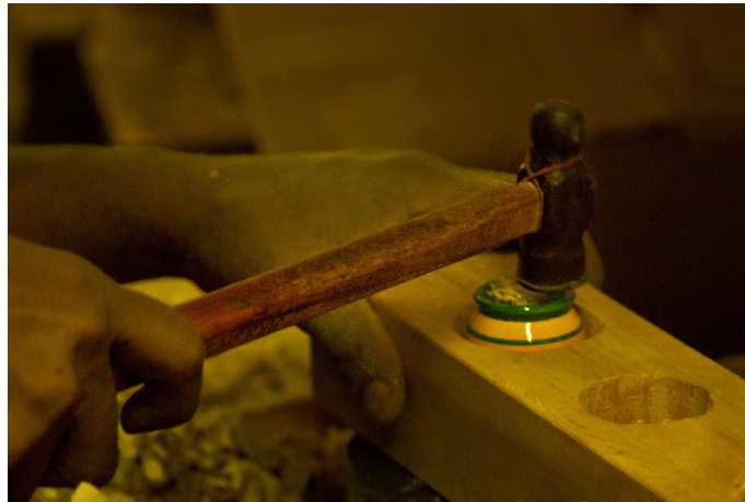
The toy is fixed in the wooden jig.
