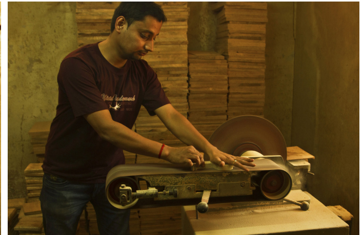
Sanding process levels the wooden surface.
