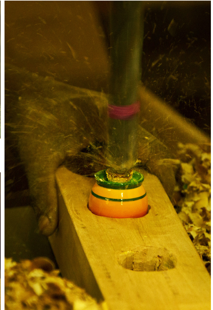
Hollow space is created to reduce the weight in the toy.
