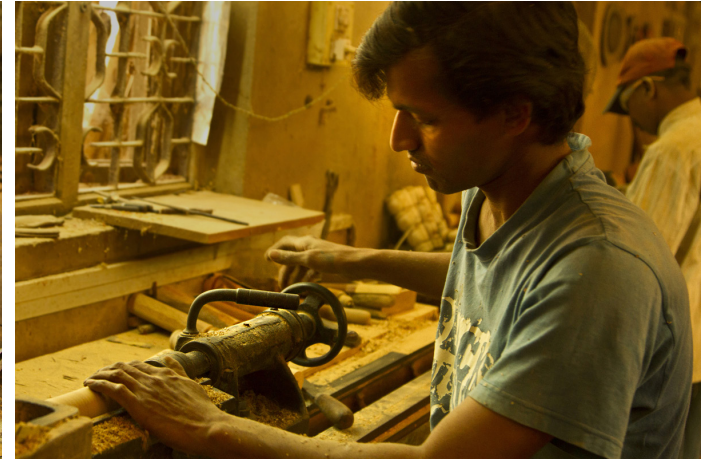
Wood turning machine is used for faster productivity and time saving.
