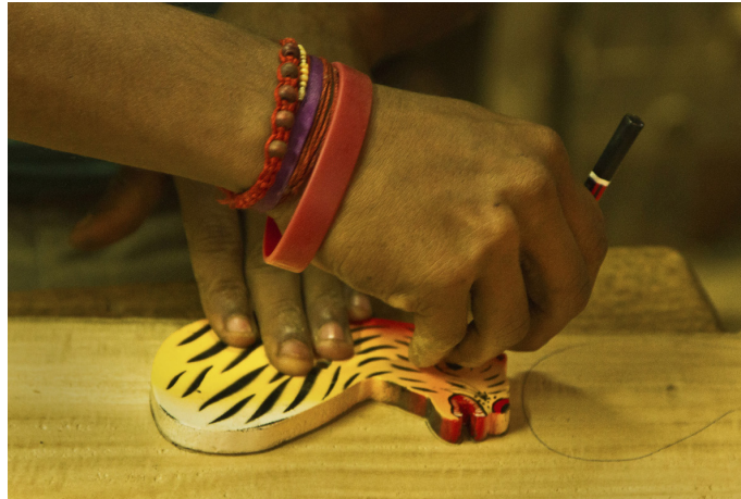
With the help of a masterpiece, shape of the toy is marked on the wooden plank.
