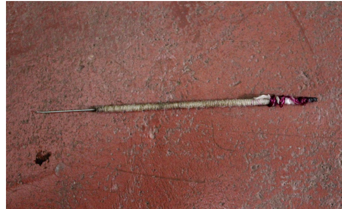
Needle for pulling out the thread that goes back and forth of the fabric while making embroidery.
