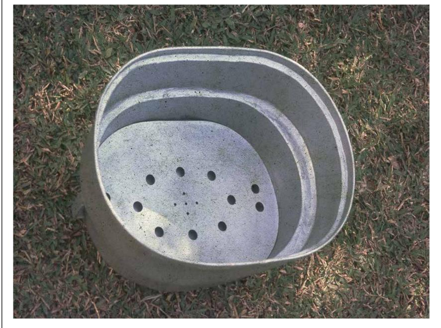
Prototype of 2nd solution was also made in stainless steel and painted with aluminum paint. A drainage for water was provided in bothh solutions
