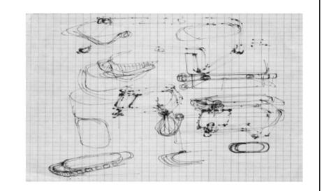
We also developed an alternative design in elliptical shape. This had a step with wide opening. Big fish could be carried easily in this. Injection moulding or Rotomoulding would have been better options for the elliptical basket. Aluminum was suggested considering the feel of hygiene it can offer! It had to be deep drawn in aluminum for production. Tooling costs would be high if it is not made in larger numbers.
