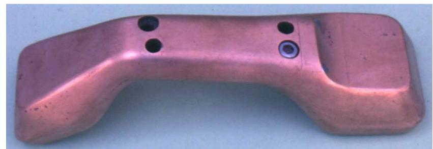
Making Moulds for injection moulding became a complex task for small scale tool makers, who had taken the contract! They were not familiar with complex shapes. For spark erotion small increase in the dimensions was required. Finally I filed and finished the copper masters myself as lot of visual judgement was involved!
