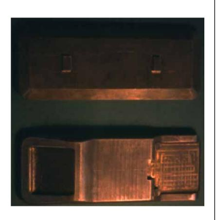
Wall mounting required a base plate. I designed the base plate for injection moulding. I also used a texture built with Cdot symbol as an element!
