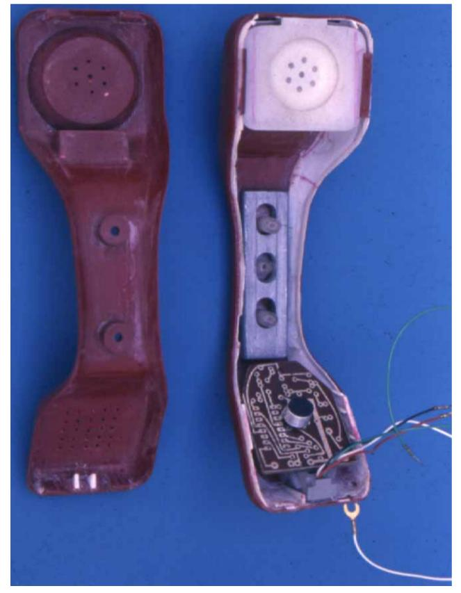
It was for the first time plastic prototypes for injection moulding were made at IDC. Our development engineer, Govinda Rajan and his team worked hard to get the details. Cutting and pasting of vaccum formed parts helped in achieving thickness variation in the edges.
